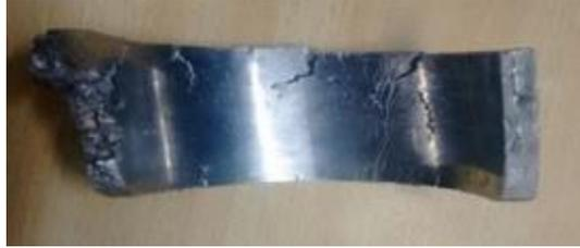
**Figure 2:** The specimen showing the Aluminum copper metal matrix composite before rolling.
